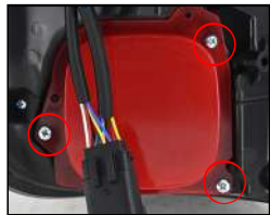
1. Remove the 3 screws. 移除3颗螺丝
