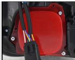
6. Press firmly to tighten the cover bracket and tighten the cover screws. 压紧盖子支架, 并将盖子螺丝拧紧
