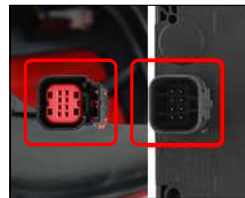
5. Insert the blind spot module connector and install. 插入盲点模块连接器并安装
